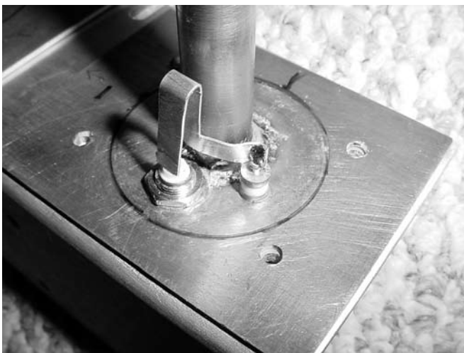
Photo A — This close-up view shows the assembly of one copper-clad circuit board material end plate with the copper pipe for L1 soldered to the circuit board, the BNC connector, copper flashing loop for L2 and the notch-adjust capacitor, C2, installed.
