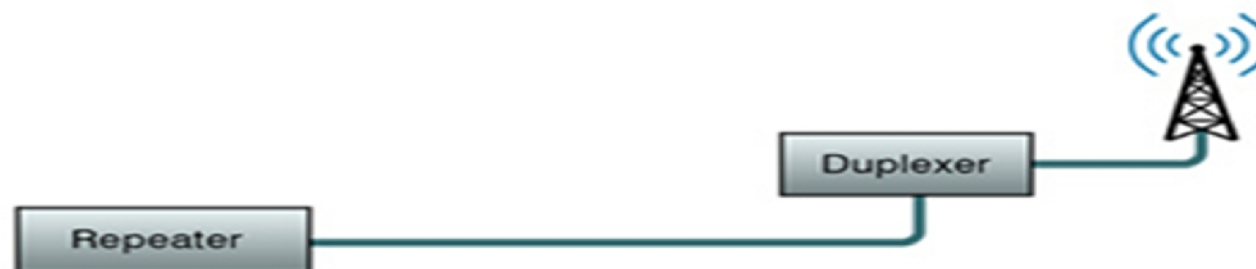
Repeater Equipment for Two Channel DMR
